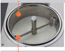
It is a real "technological pot" with a very large bottom surface area thanks to the ratio between diameter and depth. Thermal exchange is optimized without burning or sticking any product inside. The stirrer is provided with a patented counter-stirrer, easily and completely dismountable. Uniform scraping system on the whole cylinder surface, easy to remove and wash.
