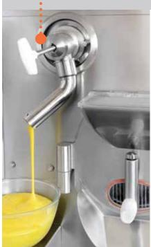
External way wide-diameter tap, working diameter 4 cm for the direct outgoing of products to the cooling cylinder, even the more dense ones, max 15 seconds for 7 kg of high density product.
