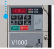
Stirrer rotation inverter working at 9 different speed levels, from 7 up to 70 Hertz. Many different products, even the most delicate, are now possible thanks to PLC and inverter as well as a perfect batch freezing depending on the produced quantities and features of the mix and on the ingredients and their mix formulation.
