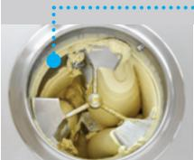
The stirrer rotation direction does not change according to speed. Therefore the machine mechanical operation is much more reliable over time.
